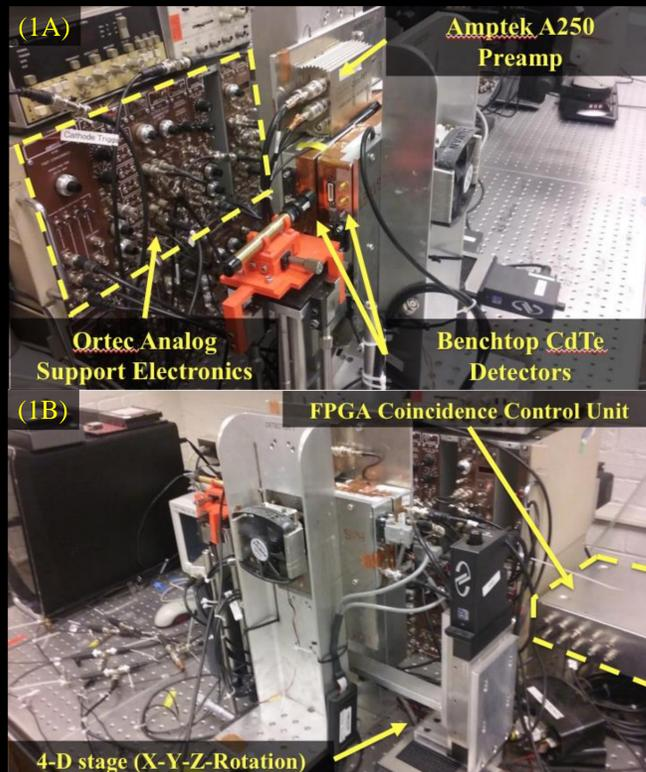
Fig. 1. (A) Ortec analog shaping and CFD electronics were used to process the Amptek A250 preamplifier signals generated from coincidence events. (B) System triggering is controlled by the FPGA coincidence control unit (Xilinx Spartan-3E). The 4-D stage used in the experiments allowed source alignment and the simulation of a multi-detector ring through rotation.
