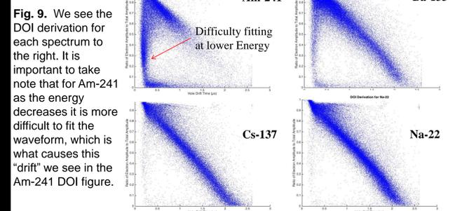
Fig. 9. We see the DOI derivation for each spectrum to the right. It is important to take note that for Am-241 as the energy decreases it is more difficult to fit the waveform, which is what causes this "drift" we see in the Am-241 DOI figure.
