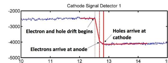
Fig. 4. (A) Digitized cathode from one of the detectors in the coincidence setup. The waveform is digitized and fitted using a linear fit method. Given the fitting it is possible to acquire the energy, depth of interaction and timing. The anode only provides the spatial position. x
